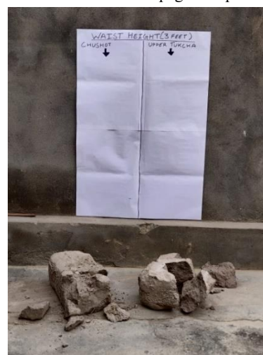
Figure 2. Comparative strength of mud brick of two spots (Chushot and Upper Tukcha)
